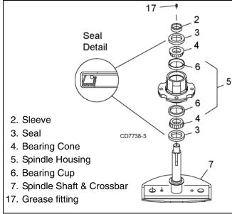
Figure 17. Spindle and Shaft Assembly
